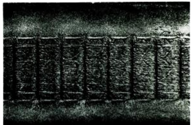
Figure 3. A greatly enlarged section of a recorded magnetic tape showing how the varying audio currents produced in the recording head have created tiny magnets in the tape coating. These magnets when run past the playback head will induce in the head coil a current that corresponds to the original current that created them during recording. The magnetic patterns are not visible to the naked eye.
